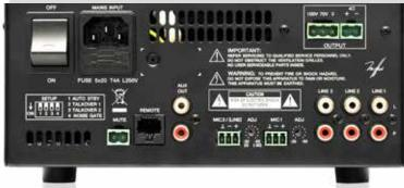
Self-powered mixer including an integrated media player and 5 external audio inputs: 3 x LINE ST, 1 MIC/LINE and 1 MIC. It features a 120W powered output that supports both low  $(4 \Omega)$  and high impedance (70V, 100V)loudspeaker lines. It also includes a 2 level priority system (paging, emergencies, etc.), auto stand-by mode, AUX OUT and an additional remote control port to manage the source selection and output volume by means of WPm series wall panels.
