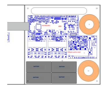
The following figure shows the battery connection to the electronic card of the power supply unit.
